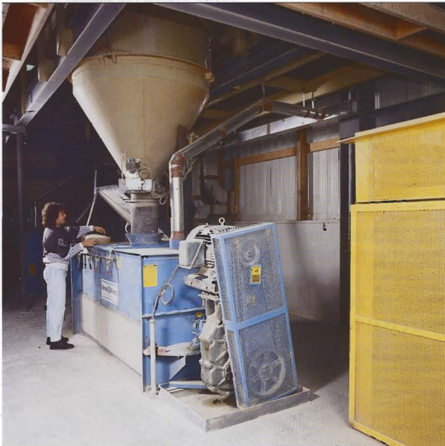
An operator adds minor ingredients to a 6,000-pound-capacity paddle mixer.
