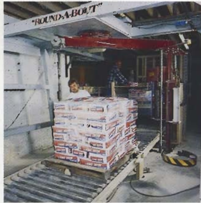
Pallets are stretch-wrapped before being loaded onto trucks or moved to a warehouse.
