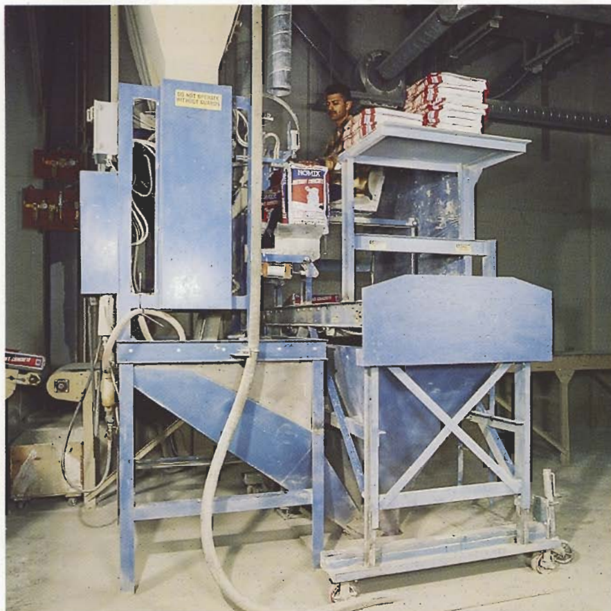
Two impeller packers for valve bags fill 60-pound bags of instant concrete.
