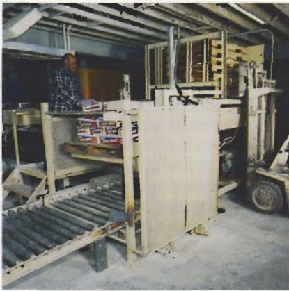
A worker arranges one layer of bags at a time on a semiautomatic palletizer.
