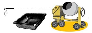
Water should then be added to bring the mixture to the proper consistency and the whole batch wet mixed. Do not use more water than is necessary as a wet mix is difficult to handle and weakens the concrete. On large jobs it is often economical to mix mechanically rather than manually. When using a mixer, the same care must be taken in weighing all ingredients and in thoroughly dry mixing to a uniform color before the water is added.
